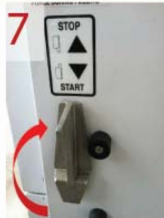
7 TURN DISPENSER SWITCH TO "STOP" POSITION
