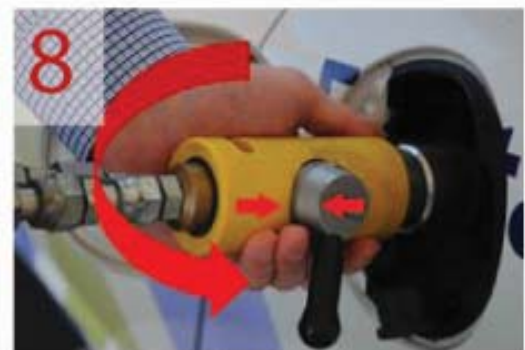
8 DISCONNECT FUELING NOZZLE (ARROWS POINTING TOWARDS EACH OTHER)
