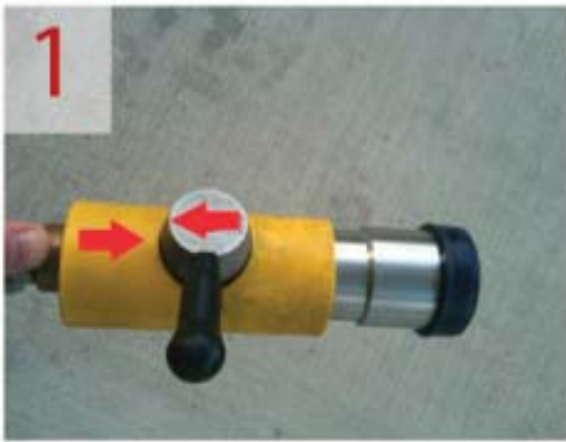
1 ENSURE FUELING NOZZLE IS OPEN (ARROWS POINTING TOWARDS EACH OTHER)
