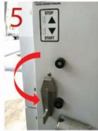
5 TURN DISPENSER SWITCH TO "START" POSITION
