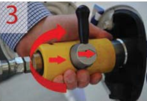
3 TURN NOZZLE HANDLE TO "FILL" POSITION (BOTH ARROWS POINTING TOWARD VEHICLE)
