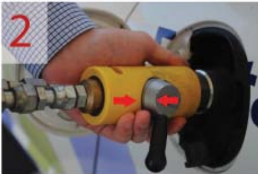
2 CONNECT FUELING NOZZLE TO VEHICLE (ARROWS POINTING TOWARDS EACH OTHER)
